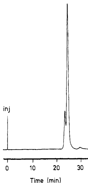
Figure 2. Partial separation of methyl pheophorbides 6 from C. ethylicum using normal-phase \mu -Porasil columns (2.3.9 mm i.d. \times 30 cm). Conditions: 1 mL/min of \text{CHCl}_3 , 1500 psi.
